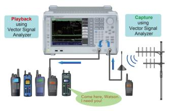
Repeatably Test Device Performance using "Real-World" RF Environments
